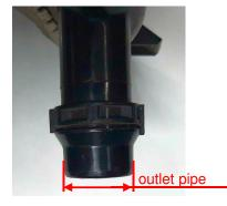
Reference outlet pipe diameter : 32.38 - 32.49 mm ADR outlet pipe diameter : 32.42 - 32.5 mm
