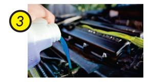
Fill the new coolant into the radiator, only use coolant that recommended by automobile company.
