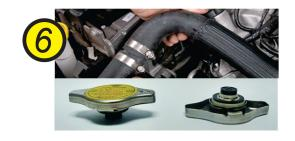
Check the important components such as filler cap and rubber hose. Filler cap must be free from rust and rubber hose must be free from leak.
